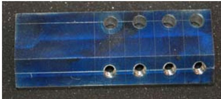
Photograph of the new mounting tabs as milled, before I cut them into separate pieces.
